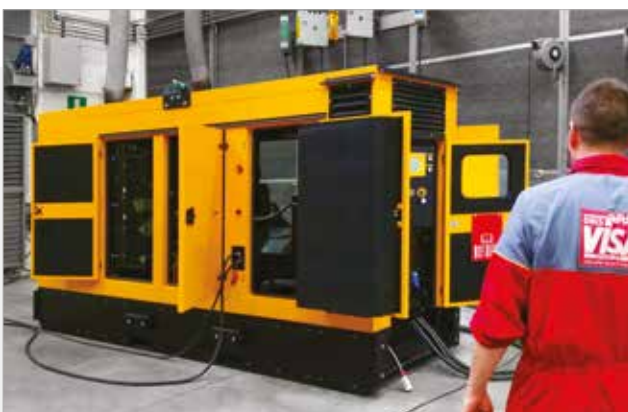
Genset soundproofed canopy
